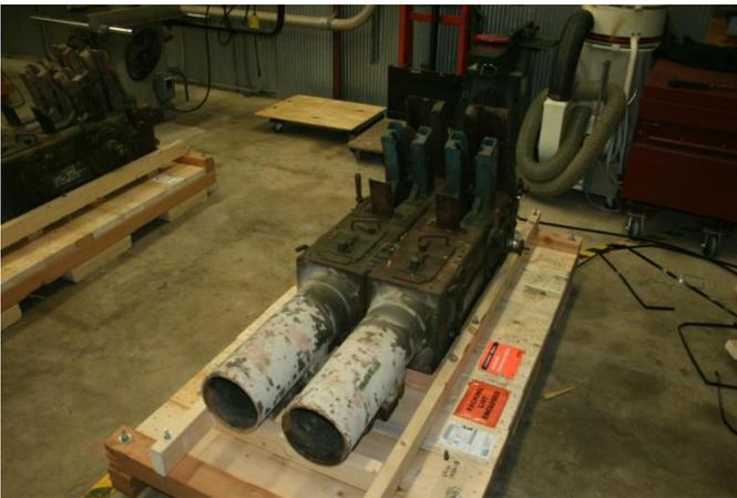
The guns were then shipped to Eglin Air Force Base for detailed inspection and modifications. Air Force Research Lab (AFRL) technicians disassembled and inspected the guns and components inspected. They found that with few exceptions, most parts were in serviceable condition. Critical parts were metal particulate inspected and re-finished with a zinc phosphate finish. Breech casings were water-blasted to
